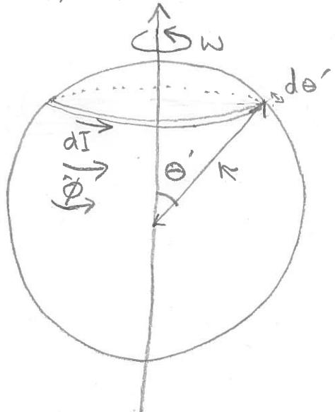
Consider surface element at angle  $\theta'$ , width  $K d\theta'$ , and speed  $v = \omega k \sin \theta'$
